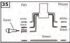
Make wiring connections as indicated above. White from fan to white from remote marked N. Blue from fan to blue from remote marked light. Black from fan to Black from remote marked L. White from house to white from remote marked AC N. Black from house to Black from remote marked AC L. Connect all green ground wires to Ground wire from House.
